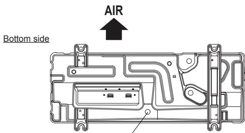
Since the drain water flows out of the outdoor unit during heating operation, install the drain pipe and connect it to a commercial 16 mm hose. (Reverse cycle model only)
