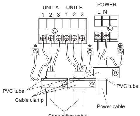
(3) As illustrated below, draw out the power cable and the connection cable.
