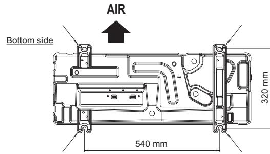
Fix securely with bolts on a solid block. (Use 4 sets of commercially available M10 bolt, nut and washer.)
