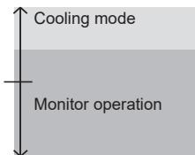
When Auto mode is first selected, the fan will operate at low speed for about a few minutes, during which time the indoor unit detects the room conditions and selects the operation mode.
